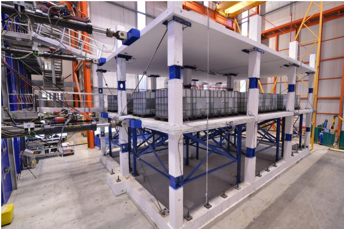
Figure 1. Test specimen: a two-storey flat slab structure
