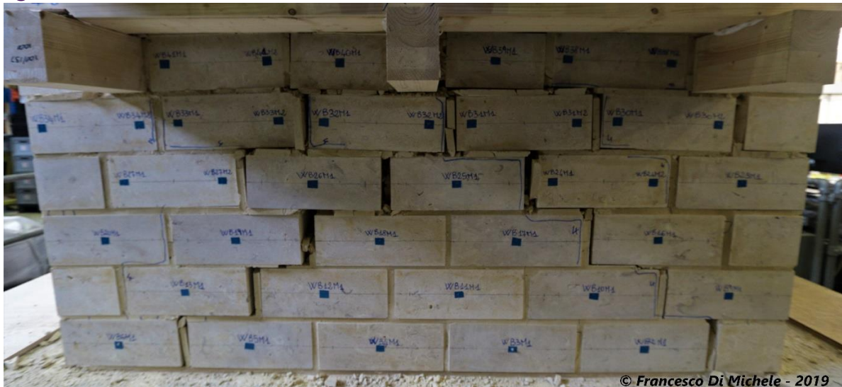
Fig.1 Typical masonry wall specimen tested.
