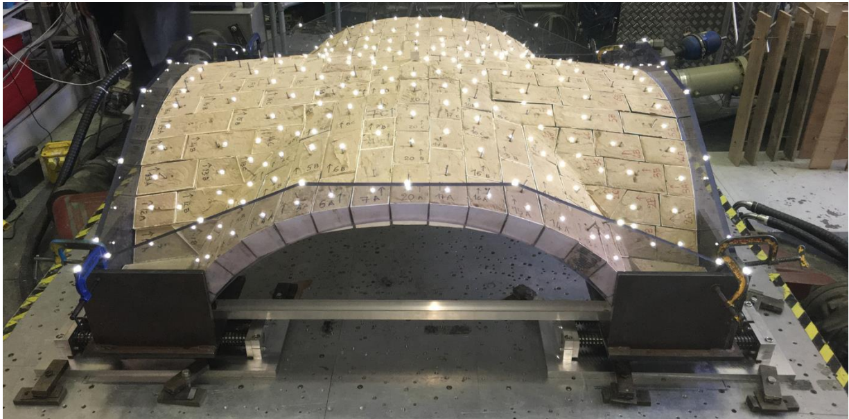
Fig.1 The vault specimen tested on the shaking table
