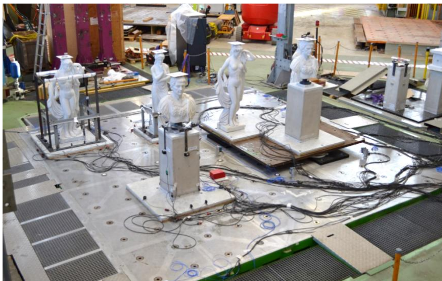
Figure 1. General set up of the statues and busts on the shake table
