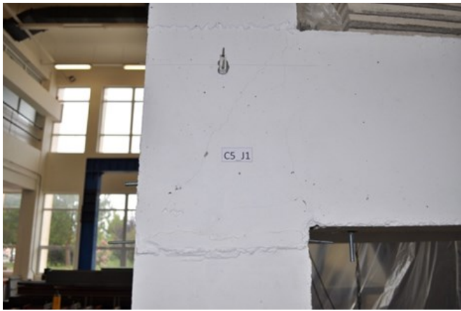
Observed damage after first cyclic test
