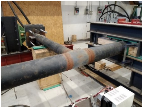
Tee joint from the tank-piping system under study
