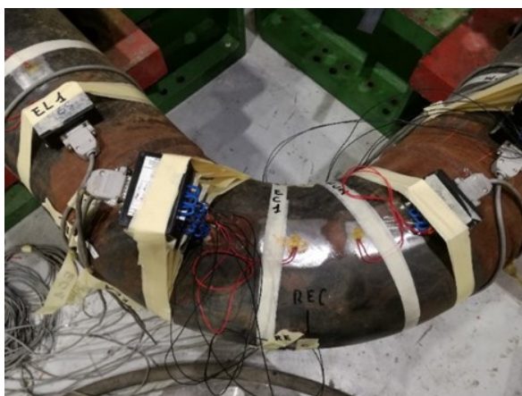
Piping elbow from the tank-piping system under study
