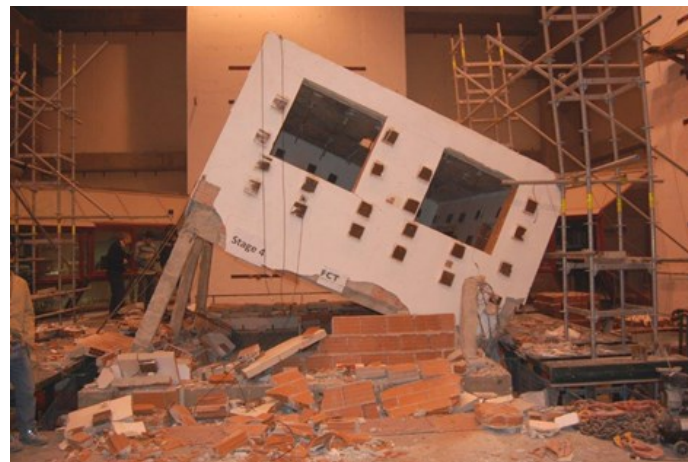
Collapse state of reinforced concrete specimen with masonry infills
