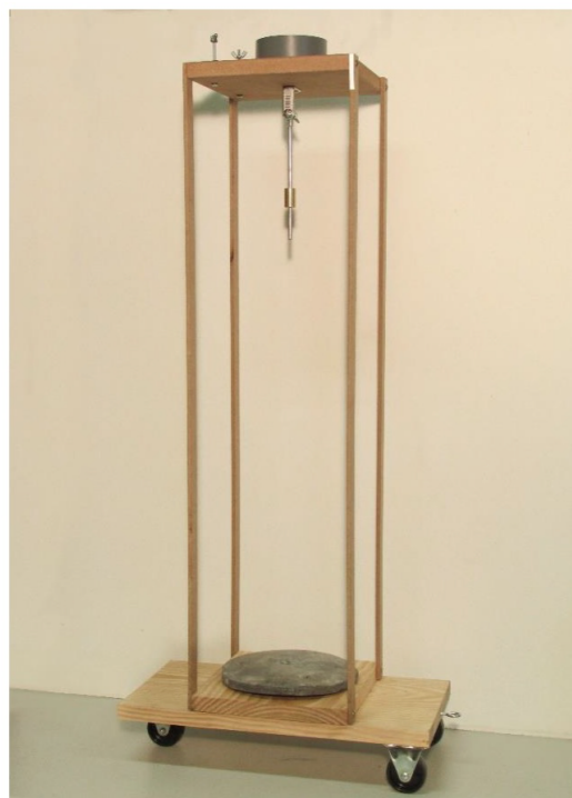
Figure 25 Tuned mass damper model, built by a 3rd year bachelor student - Raquel Pontes.
