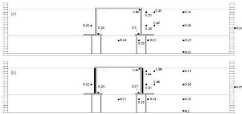
Figure 1. Maximum accelerations recorded by the sensors positioned in the backfill soil and on the bridge; comparison between two cases with piles connected to the foundation: without (a) and with (b) compressible inclusion layer behind the abutment wall (adapted from Fiorentino et al. 2019b)
