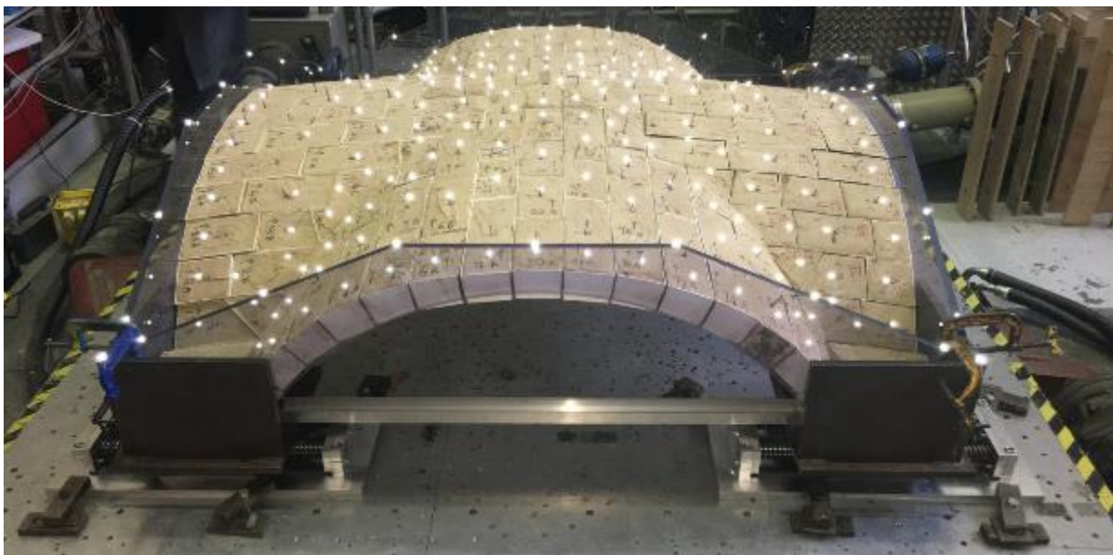
Figure 1. The vault specimen tested on the shaking table
