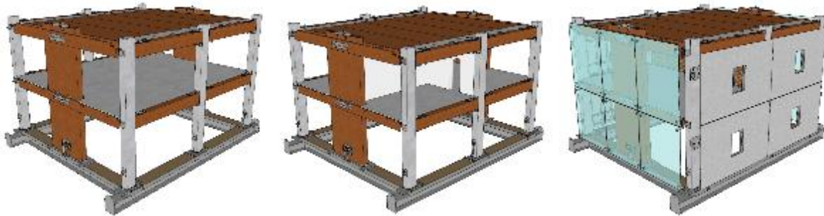
Test specimen configurations for the 3 shaking table tests performed
